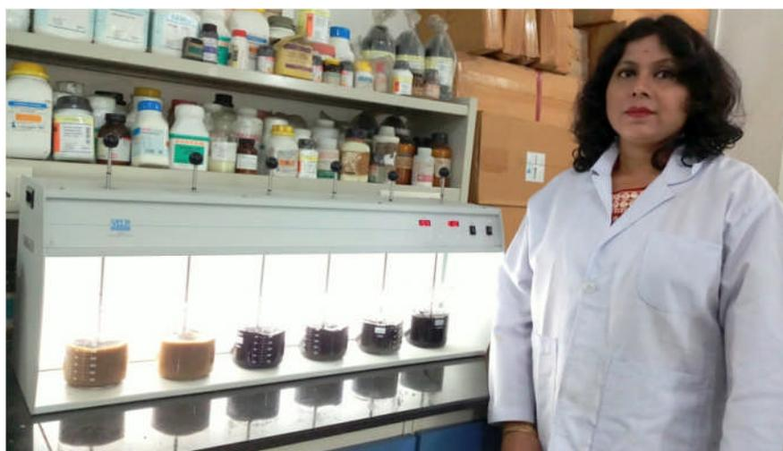
Figure 2.4.3: Leaching apparatus used for stirring of experimental samples
